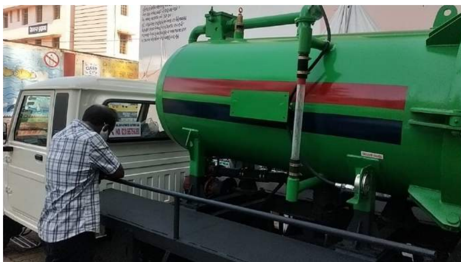
Figure 5: Small cesspool vehicle as a solution that can cater to 35 of the left out Indian population
