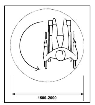
Figure 3-4: Turning radius
