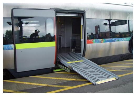
Figure 11-12: Retrofitting of ramp for sub-urban rail
