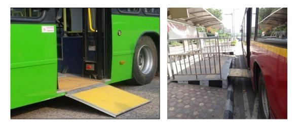
Figure 11-7: Low floor bus boarding from road level and bus stand platform
