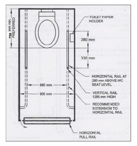
Figure 8-3: Suggested Plan WC Compartment for the Ambulant Disabled
