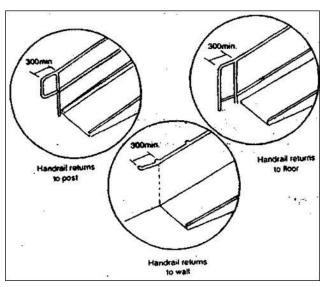
Figure 7-6: Typical handrail extensions
