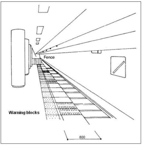
Figure 10-6: Warning blocks on platform edges
