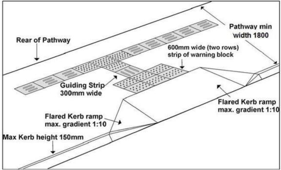
Figure 7-1: Kerb ramp detail
