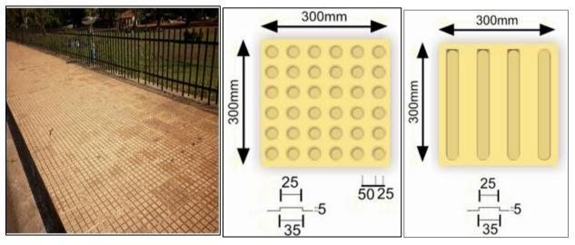
Figure 5-1: Chequered tile on footpath
