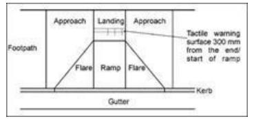
Figure 7-2: Kerb extension at street intersection
