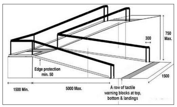
Figure 7-5: L-shape ramp with landing
