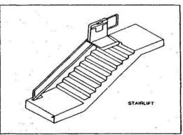
Platform lifts can have either a vertical or an inclined movement.
