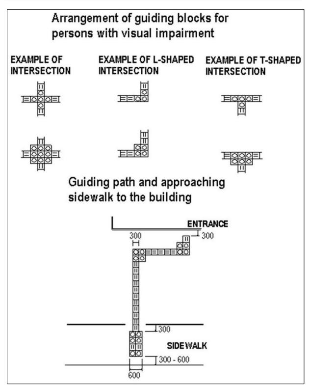
Figure 5-2: Configuration and layout of tactile pavers: guiding and warning
