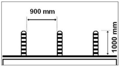
Figure 5-3: Bollards with spacing for wheelchair users/prams
