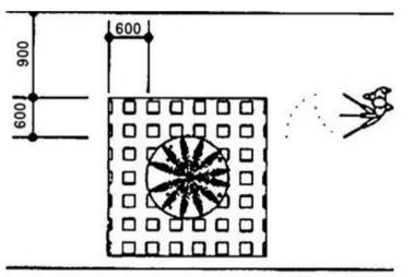
Figure 5-6: Placement of obstacles outside path of travel
