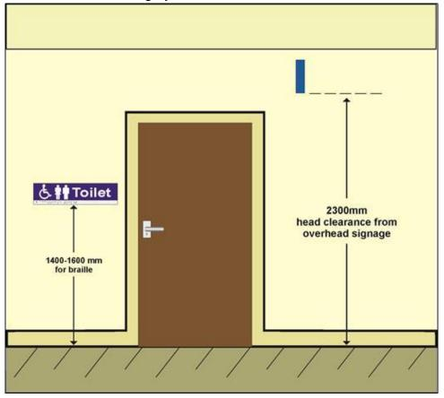
Figure 6-17: Height and placement of signages
