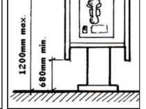
Figure 5-35: Space allowance for telephone counter
