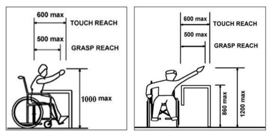
Figure 3-11: Forward and side reach over obstruction
