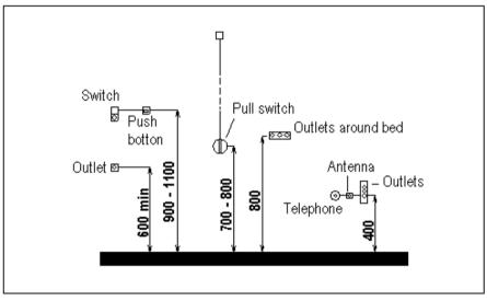
Figure 5-28: Location of electrical sockets, control, etc.
