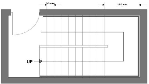
Figure 7-7: Continuous and extended handrail
