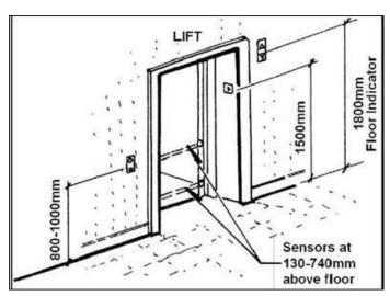
Figure 7-16: Layout of lift control panel
