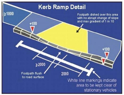
Figure 7-4: Kerb ramp detail
