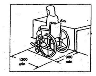
Figure 5-27: Space clearance for control operations
