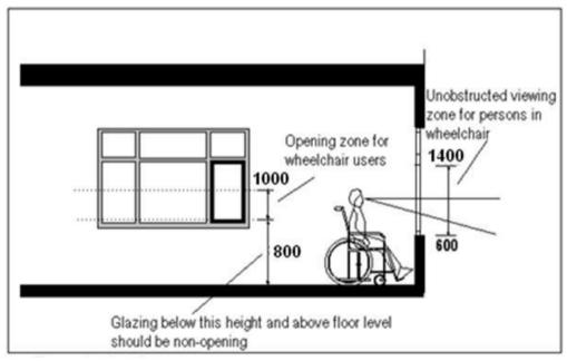
Figure 5-24: Standards for accessible window
