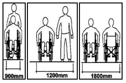
Figure 5-7: Minimum width of a clear walkway
