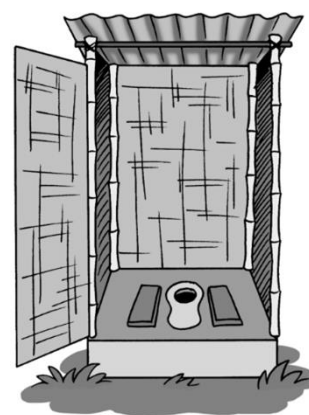
On-site sanitation technologies, like a pit latrine, will eventually fill up with fecal sludge
